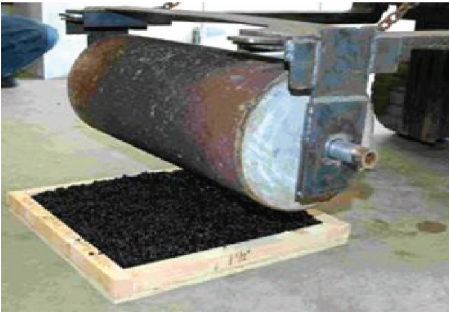
Figure 4.1 Compacting a slab for friction testing.
