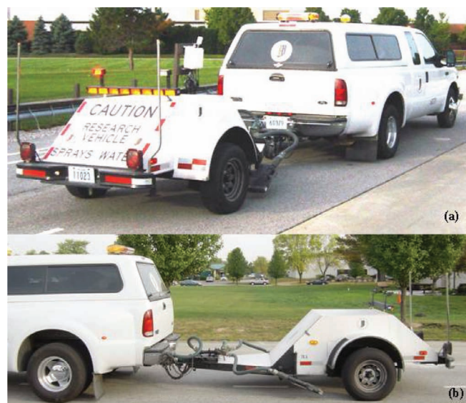
Figure G.1 ASTM E274 towed friction trailer: (a) oblique and (b) side views. (Courtesy of Kowalski, K. J. "Influence of Mixture Composition on the Noise and Frictional Characteristics of Flexible Pavements." PhD diss., Purdue University, West Lafayette, Indiana, 2007.)
